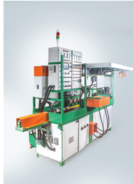
Input : 3 phase 220/415 volt AC, 50/ 60 Hz , with Neutral and Earth.
