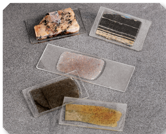
Mineral samples re-sectioned and thinned to 30\mu\text{m} .
