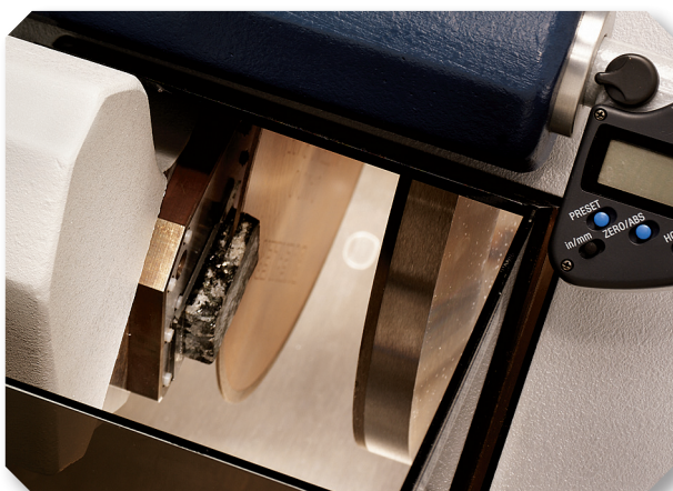
Glass slide mounted specimen resectioned on the diamond cutting blade. The grinding wheel (right) reduces the specimen thickness without having to remove the specimen after resectioning.
