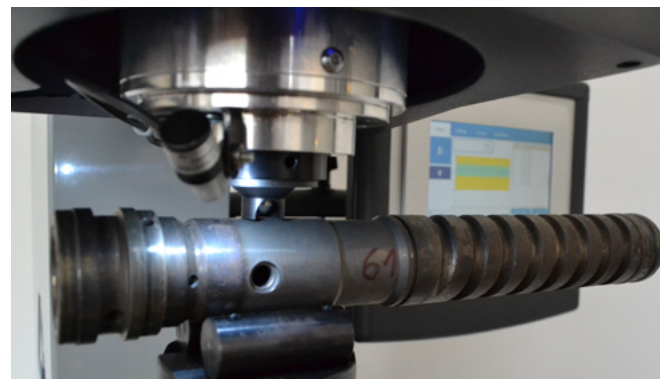
Cylindron Anvil for cylindrical parts from 50mm to 203mm in diameter. Part No. - 900007147
